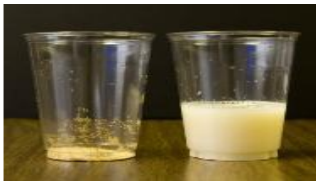
Fig 7.3: Undiluted and diluted dry flowable formulation
