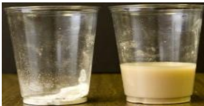
Fig 7.2: Undiluted and diluted wet table powder formulation.
