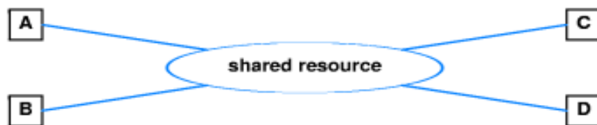
Figure 7.1 An illustration of one reason computer networks use packets. While one pair of computers communicate, others must wait.
