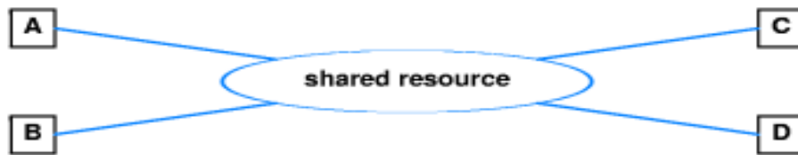
Figure 7.1 An illustration of one reason computer networks use packets. While one pair of computers communicate, others must wait.
