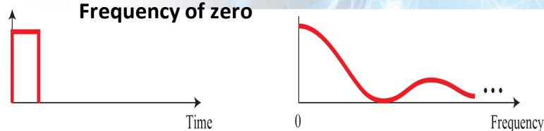
b. Time and frequency domains of nonperiodic digital signal
