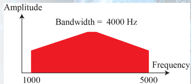
b. Bandwidth of a nonperiodic signal
